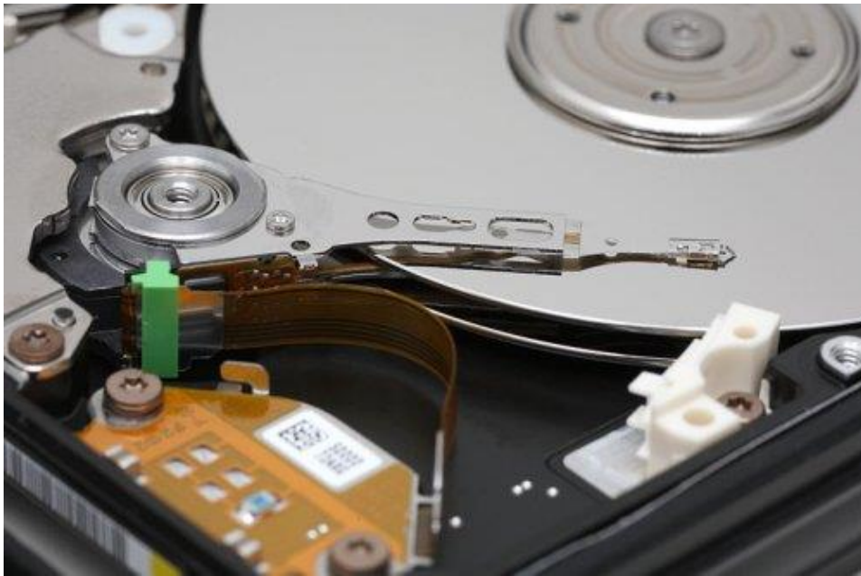
Control mechanism of the HDD head
