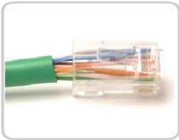
Bad connector - Wires are untwisted for too great a length.
