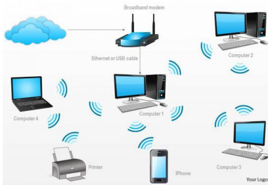
Ad Hoc Wireless Network Diagram Wireless Networking
